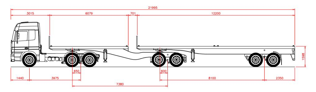
5410 = TRUCK TARE AT AXLES = 3950 7555 = GROSS MASS AT AXLES = 14925
