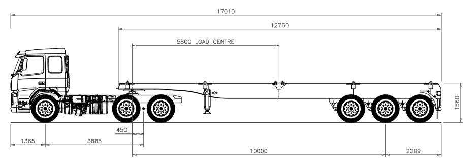
5400 = TRUCK TARE AT AXLES = 4000 7195 = GROSS MASS AT AXLES = 17695 TARE MASS AT AXLES = 4495GROSS MASS AT AXLES = 24400 (+1,6%)
