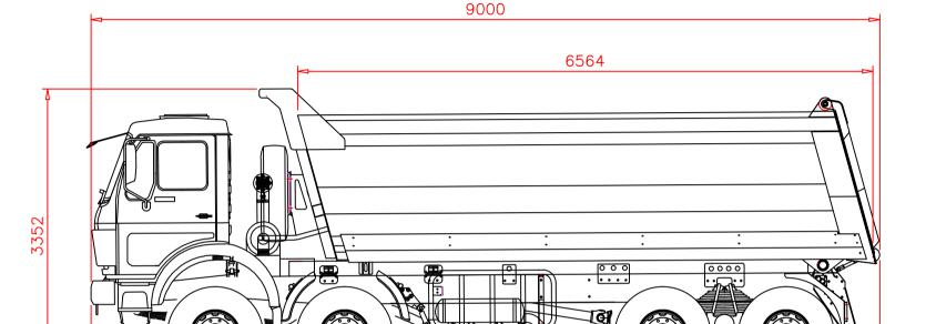
5880 = TRUCK TARE AT AXLES = 4260 12400 = GROSS MASS AT AXLES = 18500
