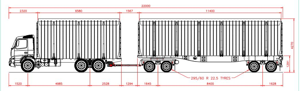
4800 = TRUCK TARE AT AXLES = 4200 7500 = GROSS MASS AT AXLES = 16500 TARE MASS AT AXLES = 3950 GROSS MASS AT AXLES = 16000
