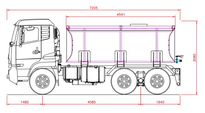
4160 = TRUCK TARE AT AXLES = 4100 7270 = GROSS MASS AT AXLES = 16490
